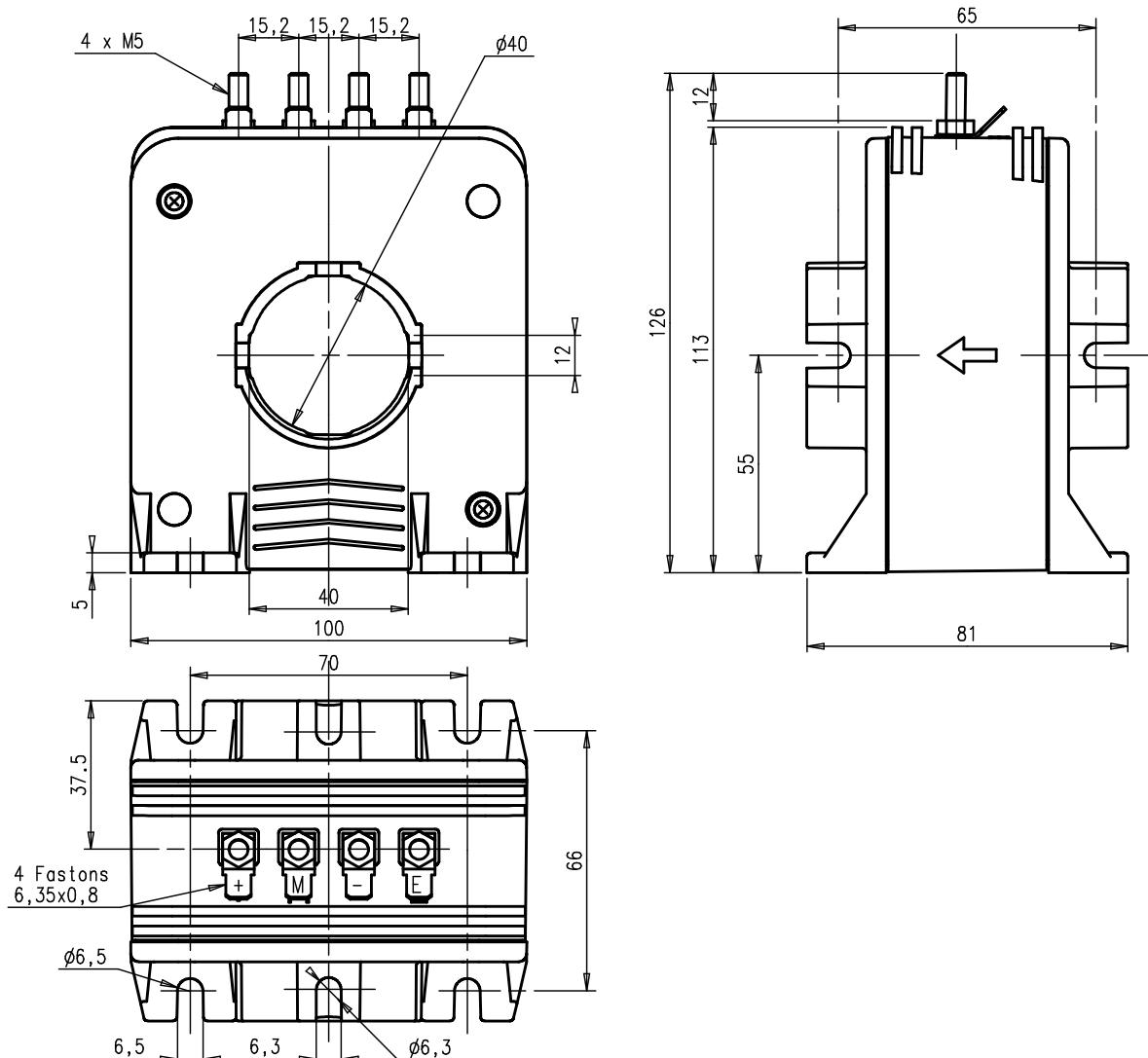
**Maximum M5 tightening torque: 2 N.m**
